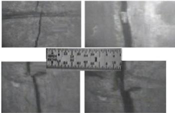
Downhole video images of hydraulically created fractures in open hole, vertical producing wells in west Texas San Andreas formation at depths of about 4500 ft (1370m).
