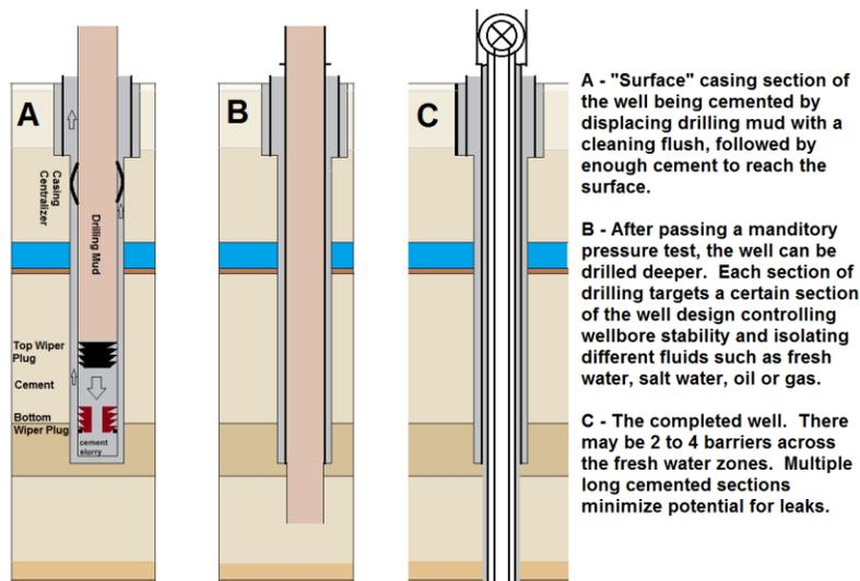
Construction of a well's barrier system begins during drilling as each casing string of the well is put in place and cemented. The completed well is a system of interactive barriers formed by steel pipe and cement. The number of barrier sets is matched to the needs of isolation for a specific section of the well.
